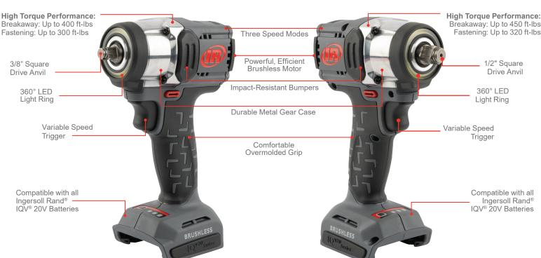
**Breakaway** Free Speed Impacts/Min Weight Length Model System **Drive Type** Light IQV® 20V Torque (ft-lbs) (bpm) lbs (kg) in (mm) (rpm) 1/2" & 3/8" COMPACT IMPACT W3131 IQV® 20V 3/8" Square 360° LED 400 2,800 4,200 2.3 (1.0) 5.2" (132) **WRENCHES** W3151 IQV® 20V 1/2" Square 360° LED 450 2.800 4.200 2.3 (1.0) 5.3" (135)
